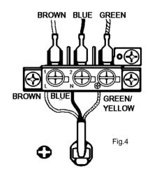
If any other type of plug is used it should incorporate a 13 amp fuse in either the plug or adapter or at the distribution board.
